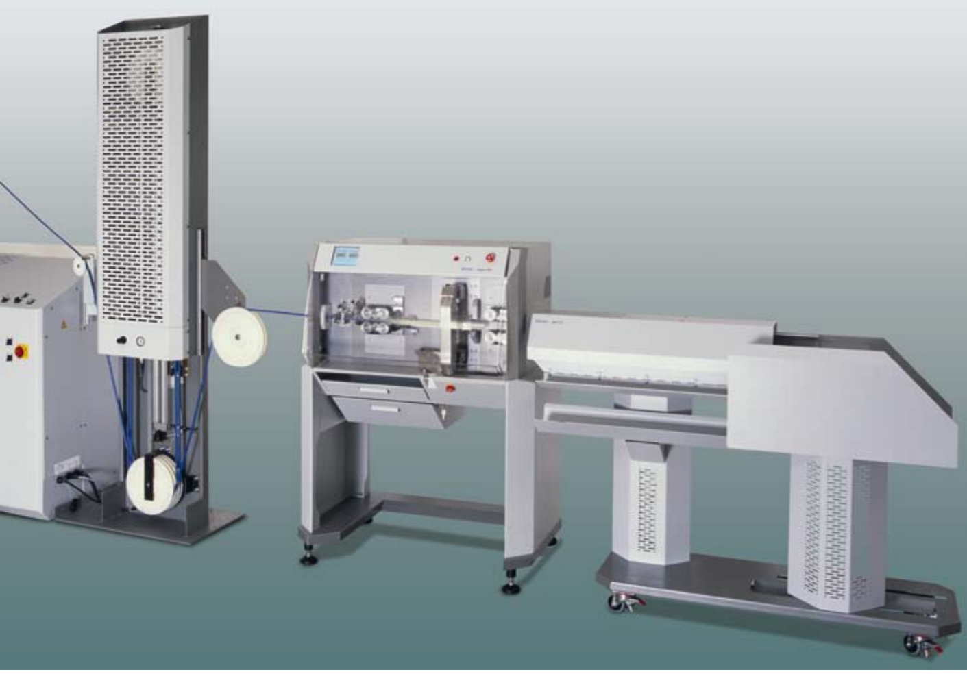
Kappa line: Kappa 350 with ads 123 feed system and dps 375 deposit system.
