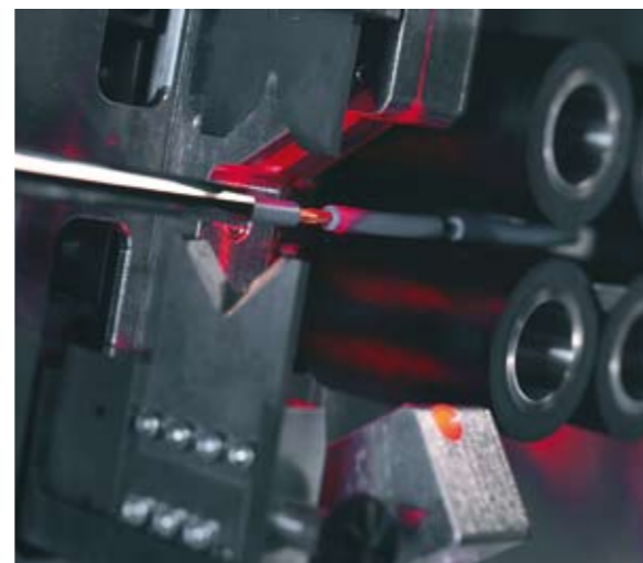
Laser sensors for cable detection
