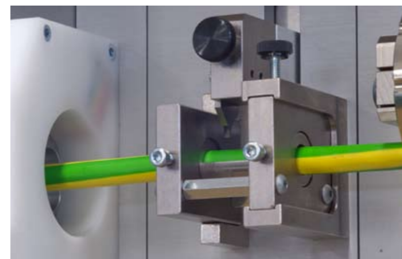
Induction and slitting unit
