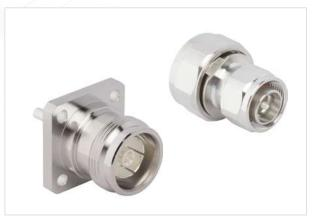
4.3-10 connectors and adapters are smaller and up to 40% lighter than 7/16 connectors, making them ideal for wireless applications. Independent electrical and mechanical planes provide excellent electrical performance and low PIM, regardless of torque.
